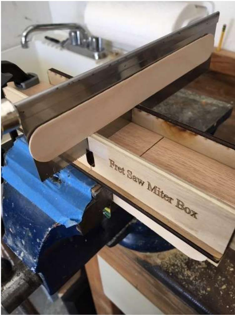
Tongue Depressor hot glued to the saw blade acts as the depth stop
