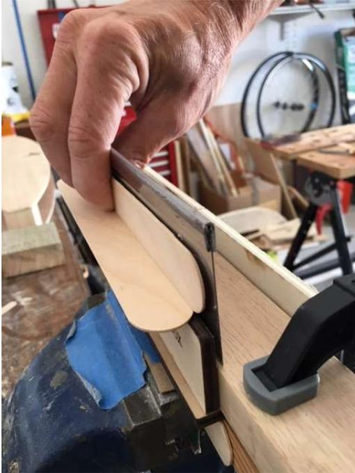
Setting the depth – saw blade resting on neck blank, tongue depressor spacing the depth stop off the top of the box while gluing the second tongue depressor to the saw blade
