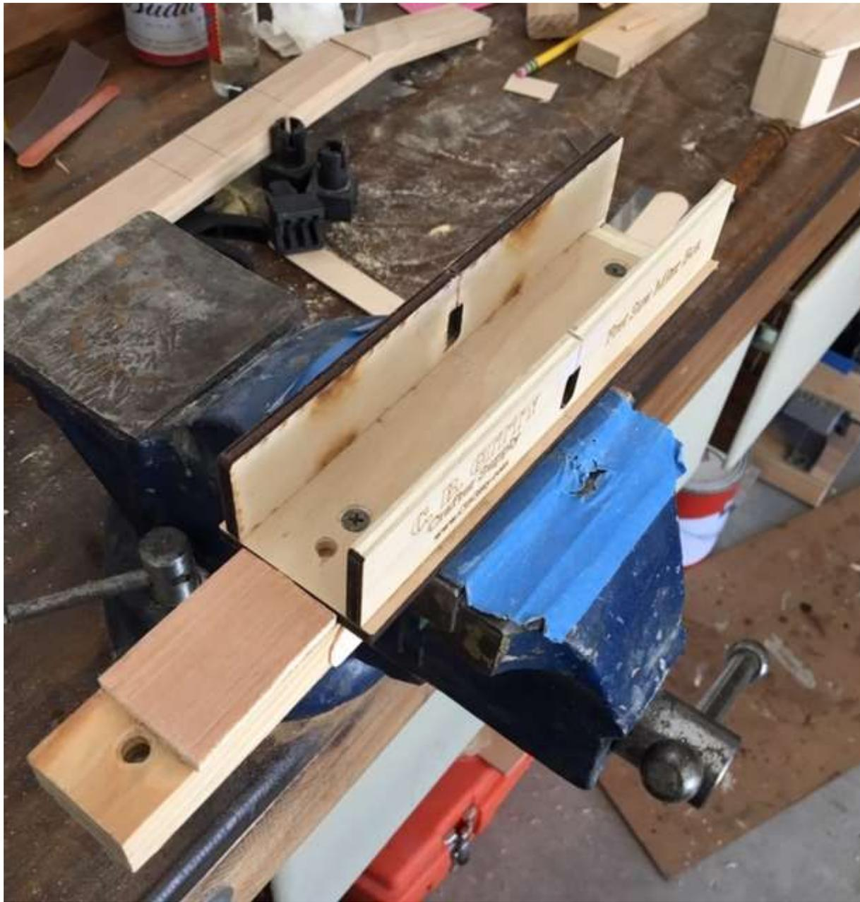
The box is screwed to a scrap of neck stock so it can be held in a vise. The extension allows the neck to be clamped while its being slotted. The shim compensates for the thickness of the box's bottom.
