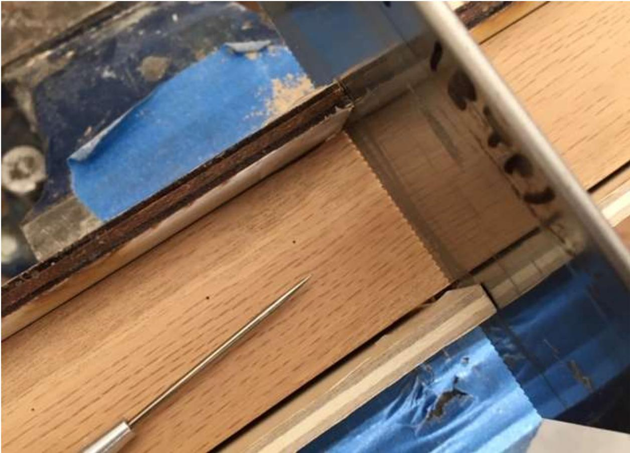
Fine awl was used to make precisely located prick marks. One mark is barely visible beneath the saw blade.
